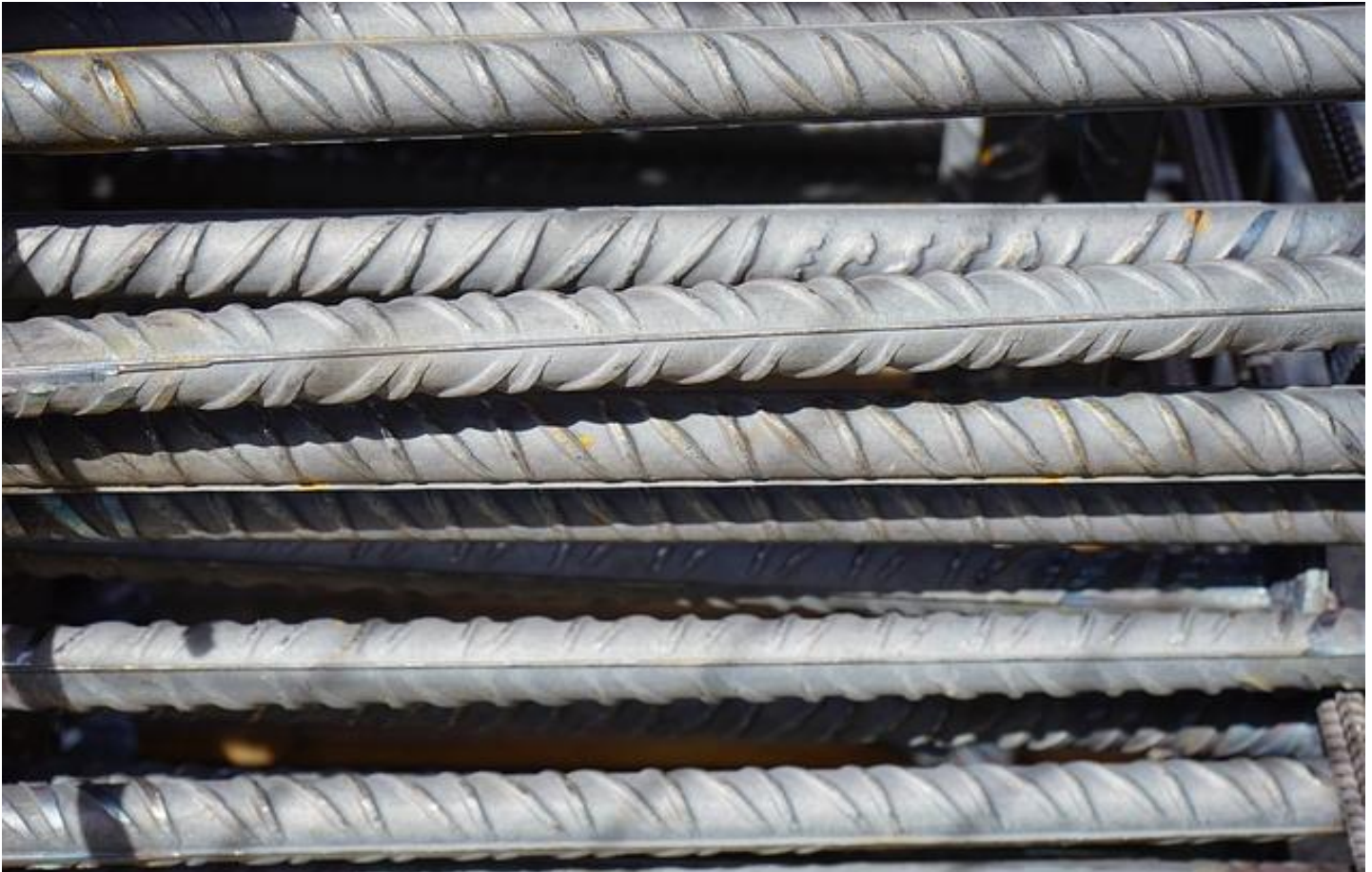
Typical reinforcement bars with ribbed protrusions.
